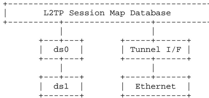
The stacking of the individual interface stacks would be described by the ifStackTable.
