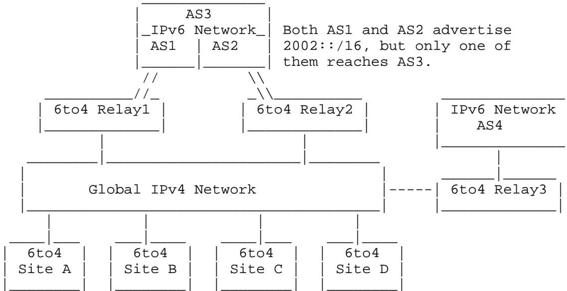
If multiple IPv6 stubs are interconnected through multiple, disjoint IPv4 networks (i.e., a fragmented IPv4 world) then the 6to4 world is also fragmented; this is the one scenario that must be avoided. It is illustrated below to show why it does not work, since the 2002::/16 advertisement from Relay1 will be invisible to Relay2, and vice versa. Sites A and B therefore have no connectivity to sites C and D.
