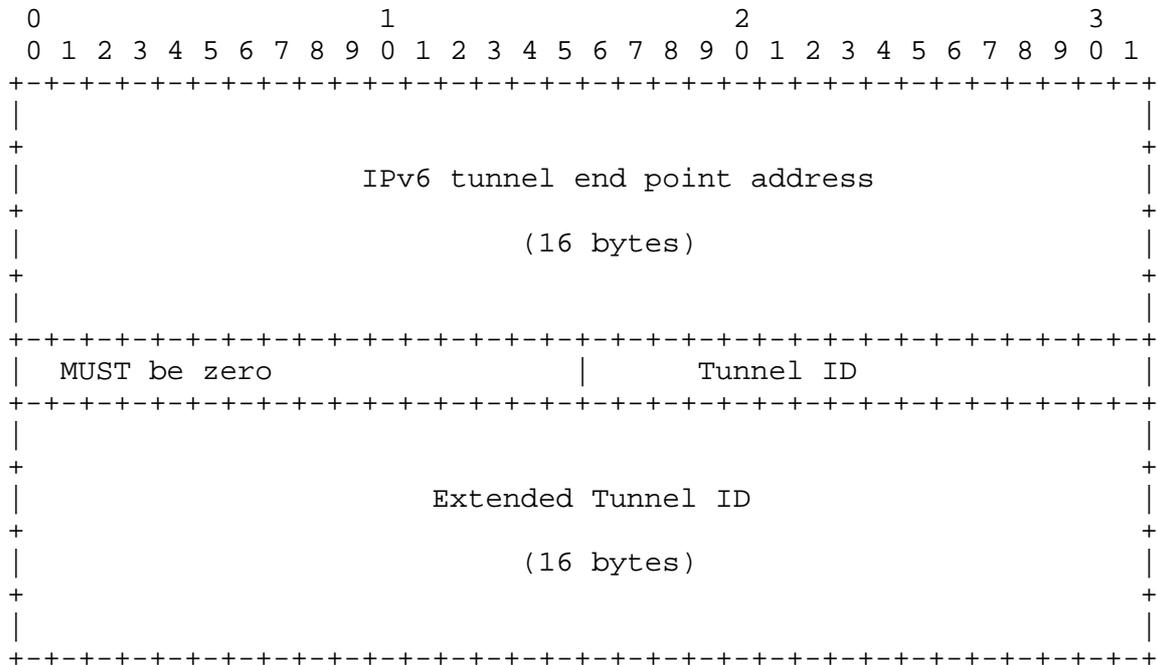
IPv6 tunnel end point address
