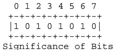
Similarly, whenever a multi-octet field represents a numeric quantity the left most bit of the whole field is the most significant bit.
