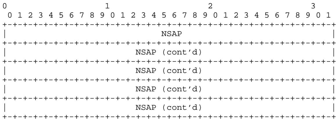
The Called Number AVP MUST be encoded as a 20 octet binary encoded NSAP address when the B bit is set in the Bearer Type AVP. The NSAP binary encoded address provides a broader range of address encapsulation methods than an ASCII field. The structure of the NSAP address (e.g., E.164, ICD, DCC) is defined in [AESA].
