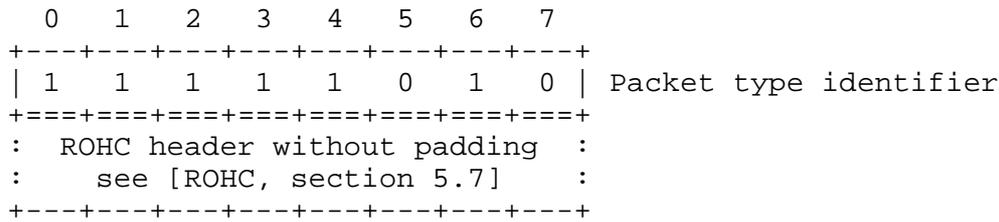
Updating properties: CSP maintains the updating properties of the ROHC header it carries.
