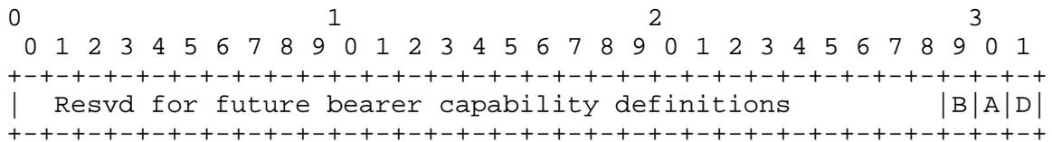
The bearer Capabilities AVP within a SCCRQ or SCCRP indicates the bearer capabilities that the sender of this message can provide for outgoing calls. This document extends the existing AVP with the B bit. If bit B is set, broadband access is supported (ATM).
