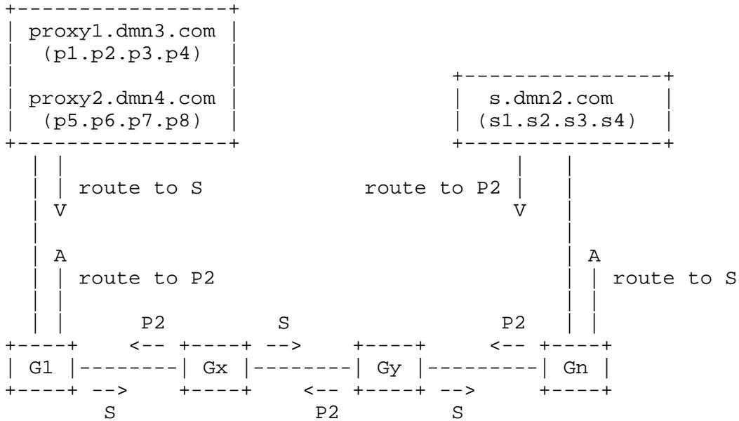
The actual FTP application work between the proxy and server is done with a bidirectional flow of TCP packets between the proxy's and server's IP addresses.
