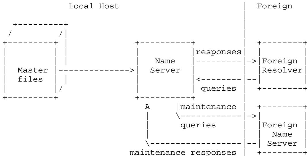
In this configuration, the name server periodically establishes a virtual circuit to a foreign name server to acquire a copy of a zone or to check that an existing copy has not changed. The messages sent for these maintenance activities follow the same form as queries and responses, but the message sequences are somewhat different.
