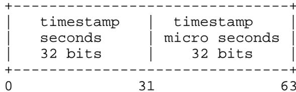
The fields are stored in XDR (external data representation) format. These 64 bits of data are then encrypted in the DES ECB mode, using the conversation key for the session. This yields:
