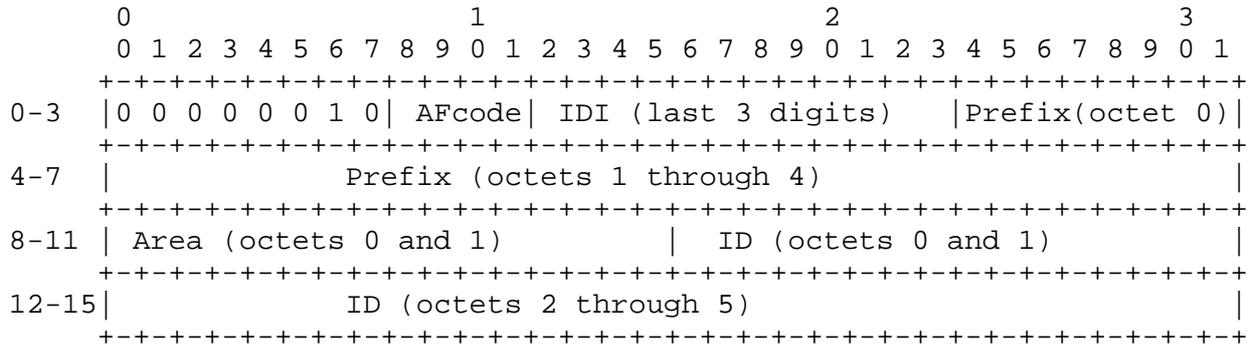
The AFcode nibble is overloaded, and encoded as follows
