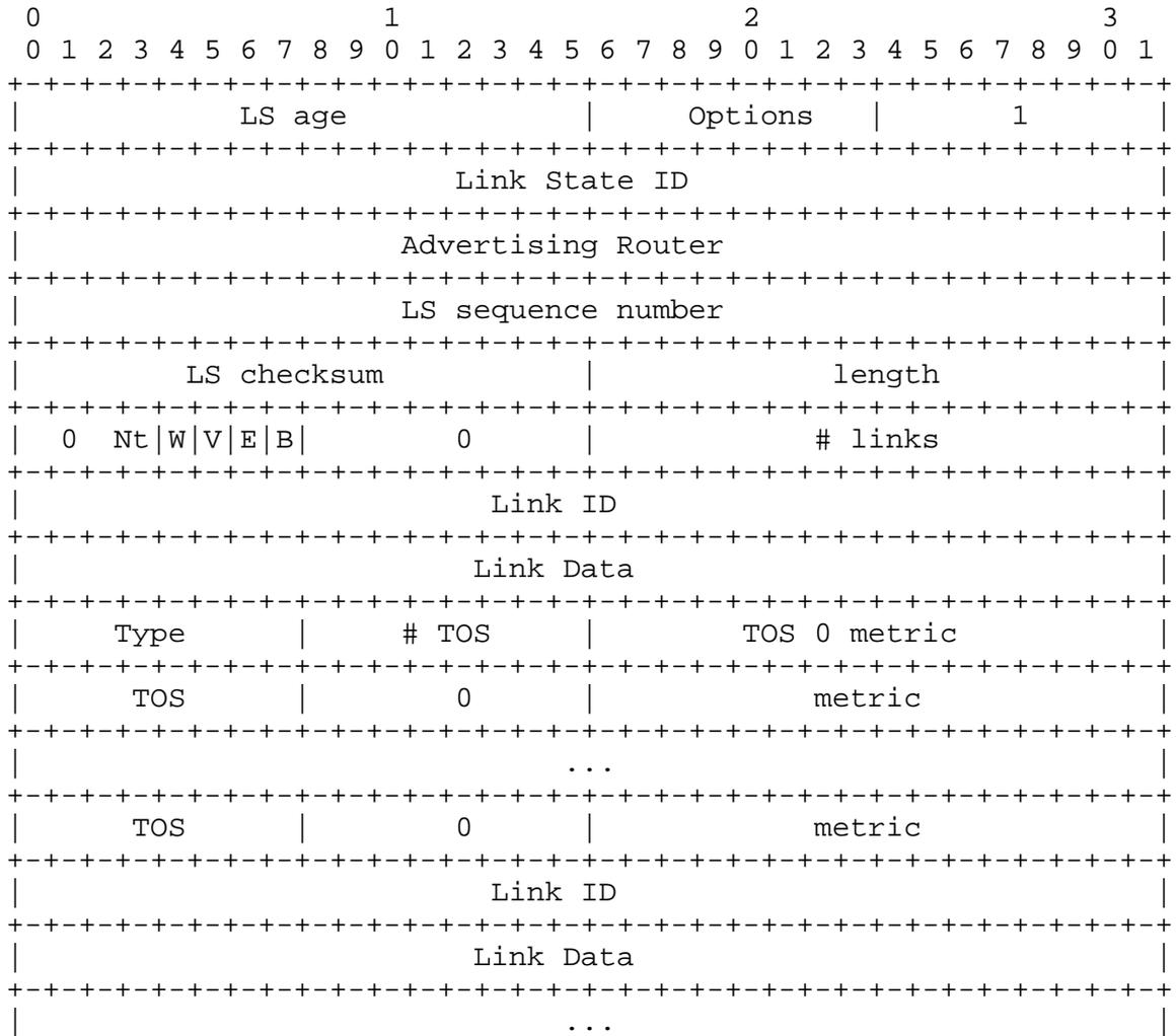
In router-LSAs, the Link State ID field is set to the router's OSPF Router ID. Router-LSAs are flooded throughout a single area only.
