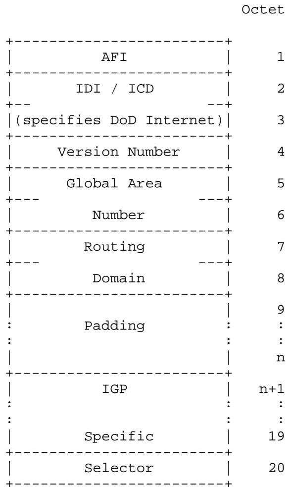
Figure 2: ISO IP address structure
