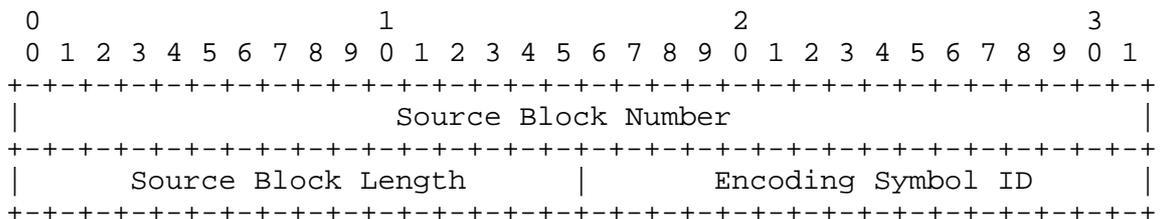
The Source Block Number identifies from which source block of the object the encoding symbol(s) in the payload are generated. These blocks are numbered consecutively from 0 to N-1, where N is the number of source blocks in the object.
