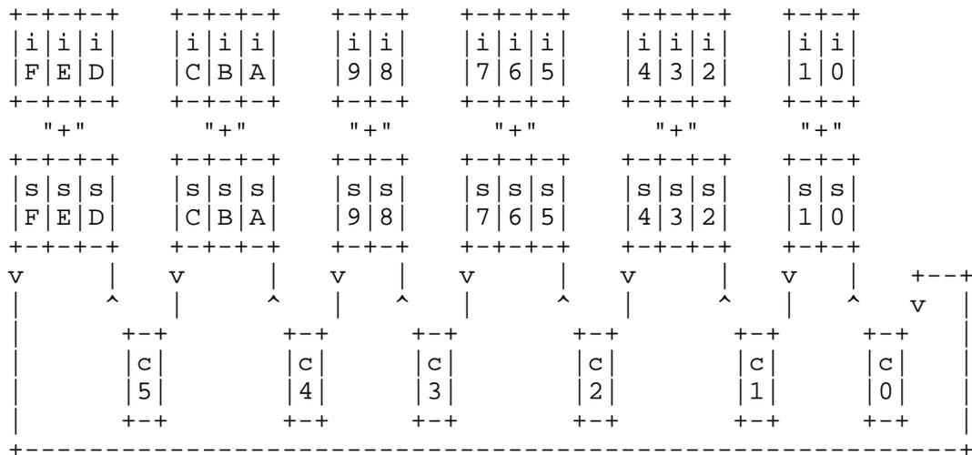
Implementation of fast-adders in PLD hardware is currently limited to 3-bits, because an i-bit adder requires  $4+2^i$  product terms, and current PLDs support only 16 product terms. The resulting device takes at most 5 "idle" clock periods for the carries to propagate through the accumulation pipeline.
