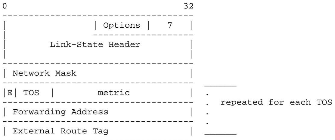
The definitions of the link-state ID, network mask, metrics and external route tag are the same as the definitions for Type-5 LSAs (See [OSPF] Appendix A.4.5), except for the forwarding address and the N/P-bit. The Options field must have the N/P bit set as described in Appendix A when the originating router desires that the external route be propagated throughout the OSPF domain.
