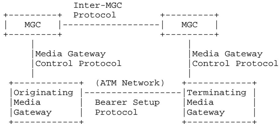
In the diagram above, the originating media gateway originates the service-level call. The terminating media gateway terminates it. In the forward bearer connection set-up model, the originating media gateway initiates bearer connection set-up. In the backward bearer connection set-up model, the terminating gateway initiates bearer connection set-up.
