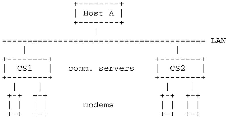
Assume that all of the modems are on the same rotary; that is, when a remote host dials in, it may be assigned a modem on either of the communication servers. Further assume that all of the remote hosts' IP addresses have the same subnet address as the servers and Host A, this in order to conserve address space.
