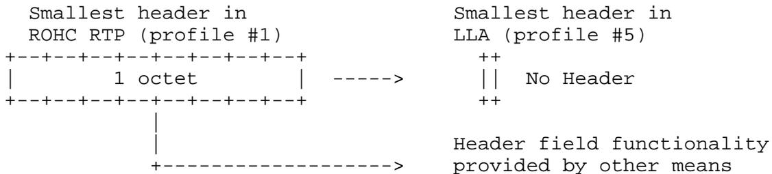
The fields present in the ROHC RTP headers for U/O-mode PT0 are the packet type identifier, the sequence number and the CRC. The subsequent sections elaborate more on how the functionality of these fields is replaced for NHP.
