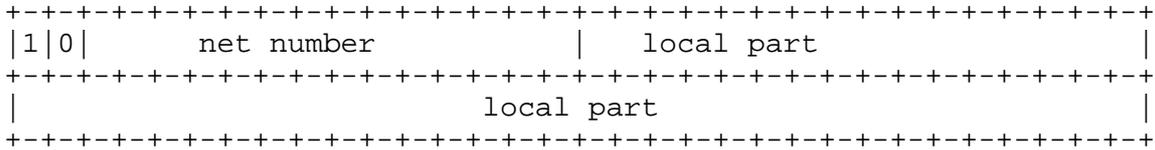
Class F-8C has the three higher order bit set to 110, a 21 bit network number and a 40 bit host address.
