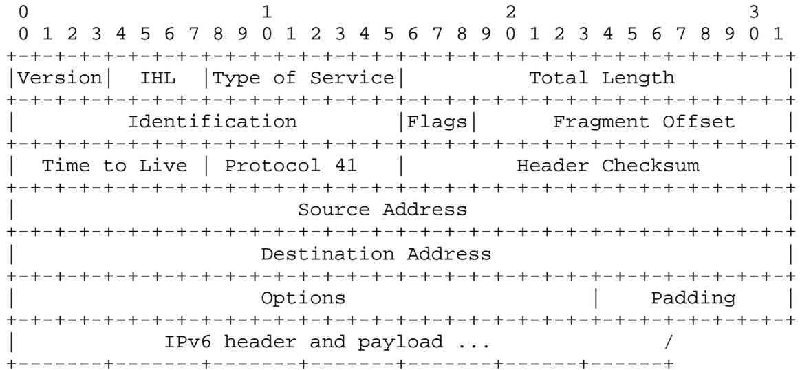
The IPv4 Time to Live will be set as normal [RFC 791], as will the encapsulated IPv6 hop limit [IPv6]. Other considerations are as described in Section 4.1.2 of [MECH].
