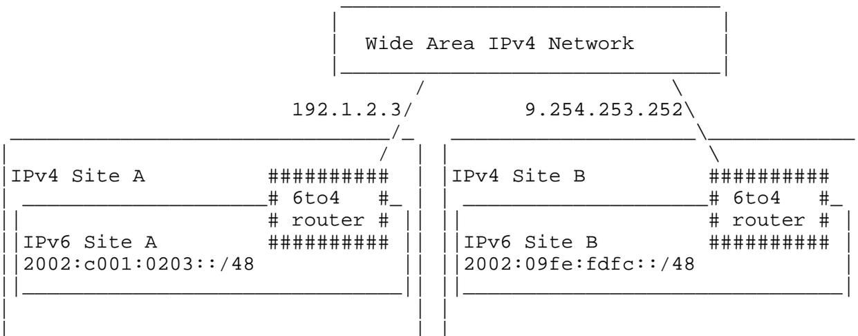
Within a 6to4 site, addresses with the 2002::/16 prefix, apart from those with the local 2002:V4ADDR::/48 prefix, will be handled like any other non-local IPv6 address, i.e., by a default or explicit route towards the 6to4 border router.
