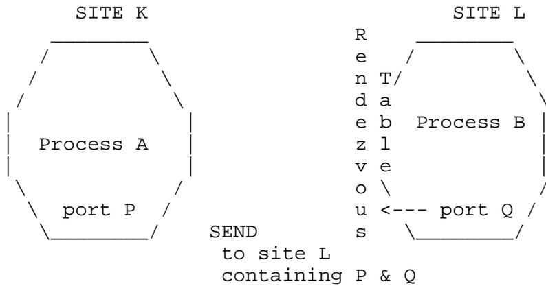
A rendezvous is made, the rendezvous table entry is cleared, and the transmission to port P at site K takes place. The SEND site number (and conceivably the SEND port number) are appended to the messages of the transmission for the edification of the receiving process.
