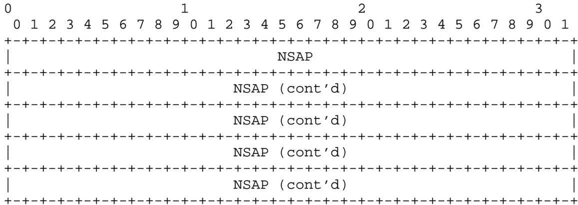
The Sub-Address AVP MUST be encoded as a 20 octet binary encoded NSAP address when the B bit is set in the Bearer Type AVP. The NSAP binary encoded address provides a broader range of address encapsulation methods than an ASCII field. The structure of the NSAP address (e.g., E.164, ICD, DCC) is defined in [AESA].
