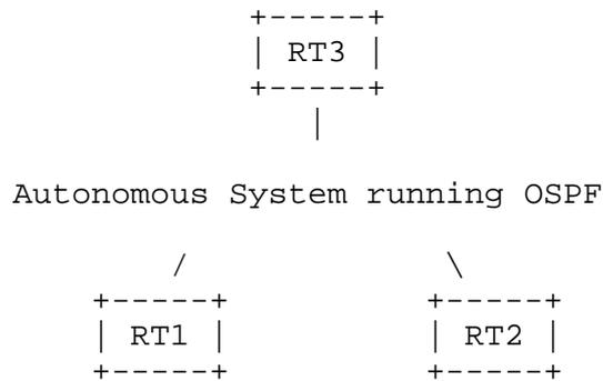
Both RT1 and RT2 have routes to an external network X and import it into the OSPF routing domain. RT3 is advertising the route to network X to other external BGP speakers. RT3 must use the OSPF router ID to determine whether it is using RT1 or RT2 to forward packets to network X and hence build the correct AS\_PATH to advertise to other external speakers.
