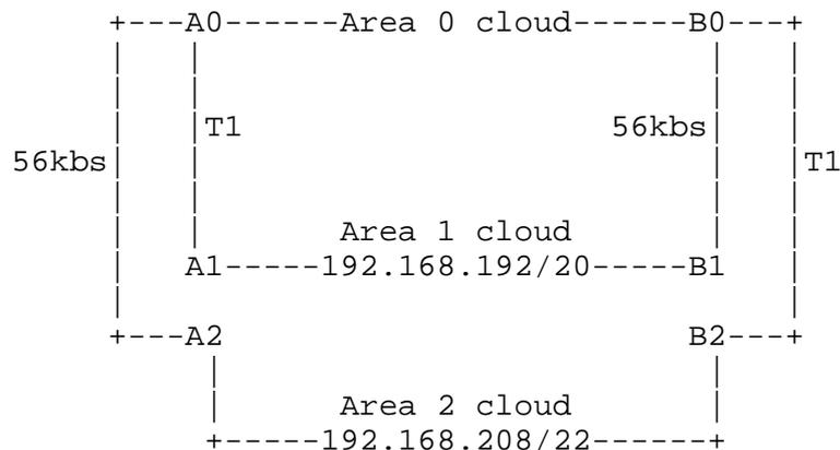
The current standard OSPF stub area has no mechanism to support the redistribution of routes for the subnets of 192.168.192/20 and 192.168.208/22 within a stub area or the ability to aggregate a range of external routes in any OSPF area. Any solution to this dilemma must also honor Area 1's path of choice to 192.168.192/20 through A0 with redundancy through B0 while at the same time honoring Area 2's path of choice to 192.168.208/20 through B0 with redundancy through A0.
