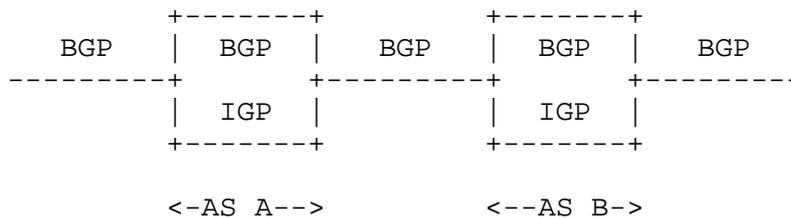
This diagram points out that, while BGP alone carries information between AS's, both BGP and an IGP may carry information across an AS. Ensuring consistency of routing information between BGP and an IGP within an AS is a significant issue and is discussed at length later in Appendix A.
