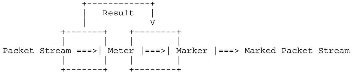
The Meter operates in one of two modes. In the Color-Blind mode, the Meter assumes that the packet stream is uncolored. In the Color-Aware mode the Meter assumes that some preceding entity has pre-colored the incoming packet stream so that each packet is either green, yellow, or red. The details of the pre-coloring process, including handling of error scenarios, and how the Meter determines the color of a pre-colored packet are DS domain specific and outside the scope of this document.
