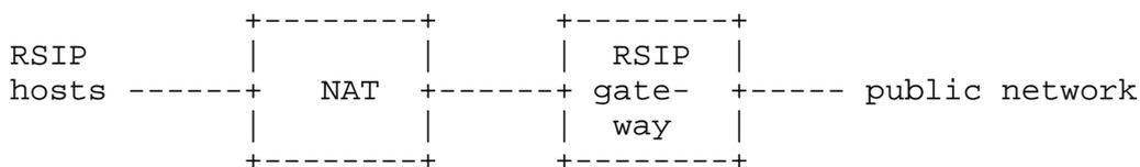
In this architecture, the RSIP hosts are separated from the RSIP gateway by a NAT. RSIP signaling may be able to pass through the NAT if an RSIP ALG is installed. The RSIP data flow, however, will have its outer IP address translated by the NAT. The NAT must not translate the port numbers in order for RSIP to work properly. Therefore, only traditional NAT will make sense in this context.
