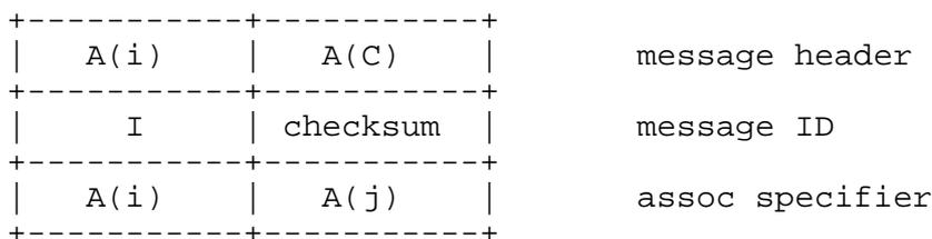
2. The Cookie Jar checks the access list to determine if the association  $[A(i),A(j)]$  is valid. If so, it rolls a random number  $K(i,j)$  and constructs the reply below. It checksums the message,
