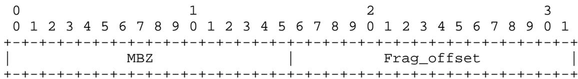
Frag\_offset: Byte offset into the audio frame for the data in this packet.
