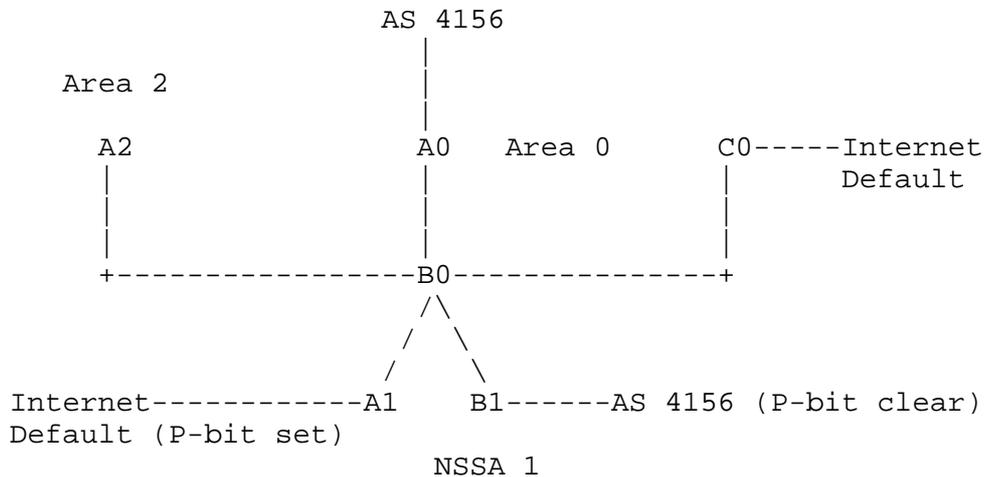
Here A0, B0, and C0 are Area 0 routers, A1 and B1 are NSSA 1 routers, and A2 is an Area 2 router. B0 is a border router for both NSSA 1 and Area 2.
