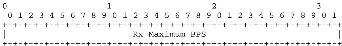
The Rx Maximum BPS is a 32 bit value indicating the speed in bits per second.
