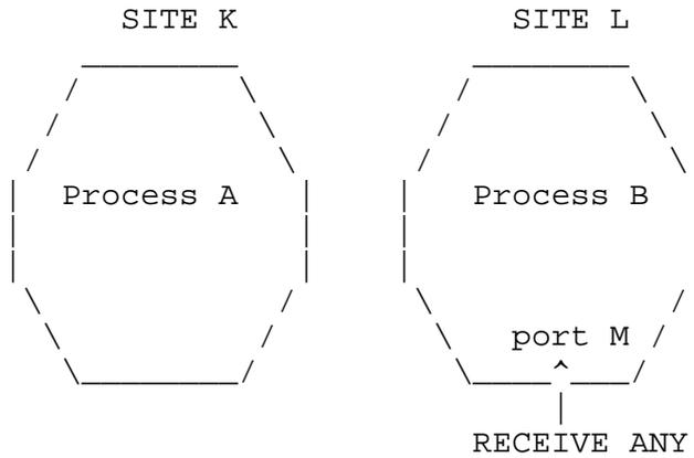
Process A, fortunately, knows of the existence of port M at site L and sends messages using the SEND FROM ANY operation from port N to port M. The message contains two port numbers and instructions for process B to SEND messages to process A to port P from port Q. Site K's site number is appended to this message along with the message's SEND port N.
