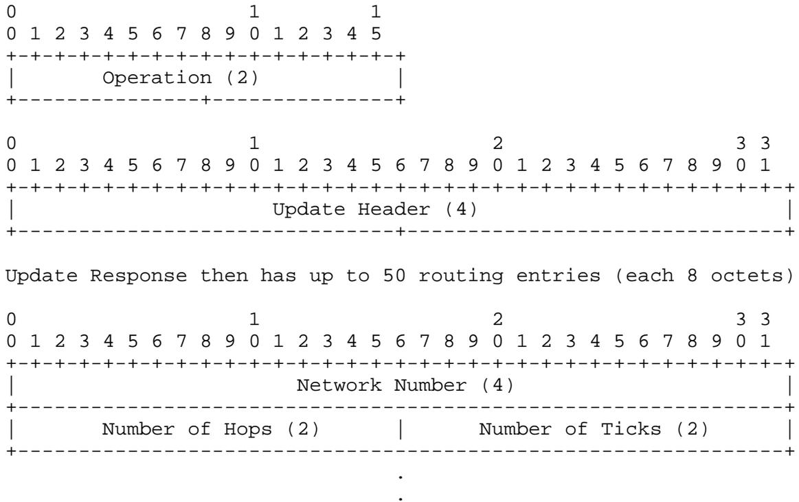
The format of a Netware RIP datagram in octets, with each tick mark representing one bit. All fields are coded in network byte order (big-endian).
