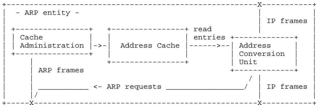
The Address Conversion Unit handles the actual conversion of IP addresses to hardware addresses. For this purpose, it uses the information in the ARP cache. The cache administration communicates with other ARP entities by ARP and creates, deletes and renews the entries in the cache.
