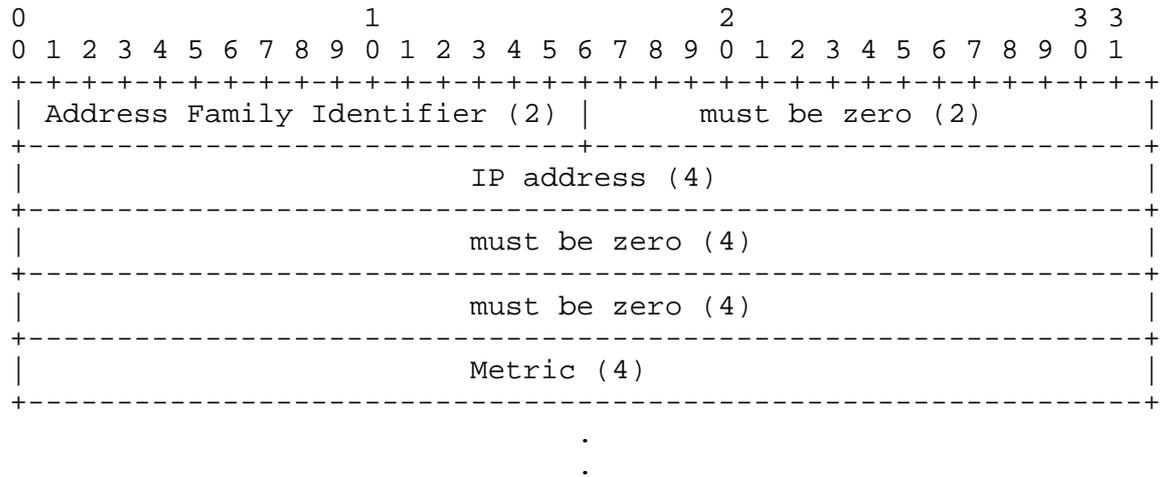
The format of an IP RIP datagram in octets, with each tick mark representing one bit. All fields are coded in network byte order (big-endian).
