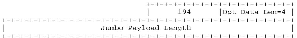
The Jumbo Payload option is used to send IPv6 packets with payloads longer than 65,535 octets. The Jumbo Payload Length is the length of the packet in octets, excluding the IPv6 header but including the Hop-by-Hop Options header; it must be greater than 65,535. If a packet is received with a Jumbo Payload option containing a Jumbo Payload Length less than or equal to 65,535,
