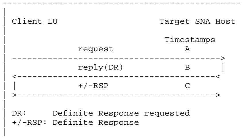
This transaction is a simple one, and is being used only to illustrate how timestamping at a target SNA host can be used to generate response times. An IBM redbook [12] provides a more detailed description of response time collection for a transaction of this type. Note that for the purpose of calculating an approximation
