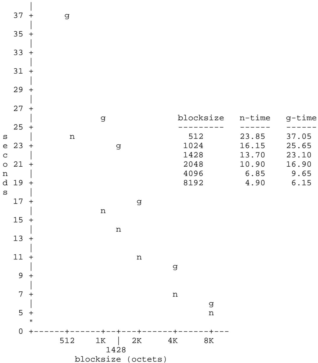
The comparisons between transfer times (without a gateway) between the standard 512-octet blocksize and the negotiated blocksize are:
