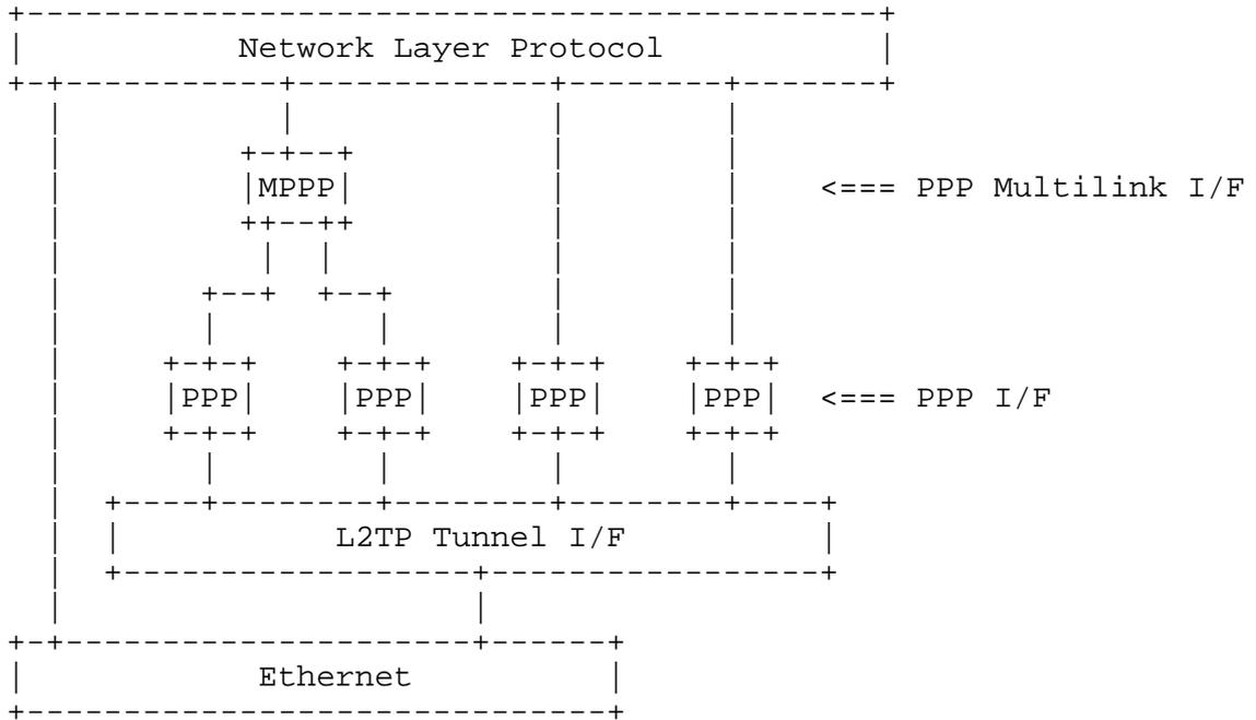
The ifStackTable is used to describe the layering of the interface sub-layers. For the example given above the ifTable and ifStackTable may appear as follows:
