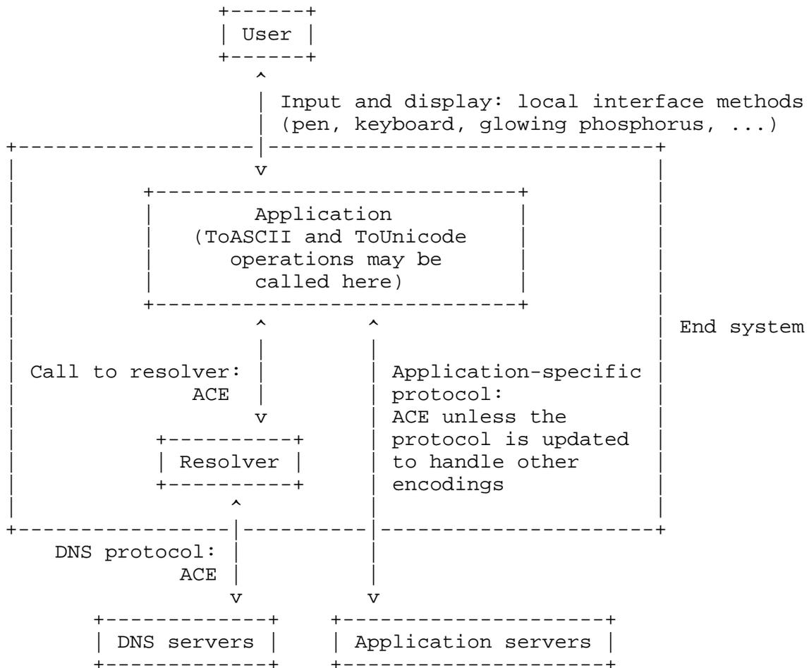
The box labeled "Application" is where the application splits a domain name into labels, sets the appropriate flags, and performs the ToASCII and ToUnicode operations. This is described in section 4.
